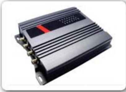
IDT 4 port reader is an intelligent high performance UHF fixed reader, which operates on 865- 867 MHz of frequency. It has an extremely high reading rate of 80- 100tags/ second, and the reading is range up to 15 meters and is antenna dependent. These readers are integrated with the antenna and are connected to a desktop PC by an Ethernet cable. The data is transferred to the PC at automatically and instantly as soon as the tags are read by the readers.
